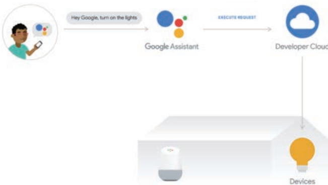
Figure 1 shows a successful fulfillment and execution of a smart home EXECUTE intent.
